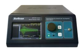
The BP-2010E features an independent operation mode, with an integrated LCD display and SD card storage, allowing for measurements and data storage without a computer connection. It also supports USB connectivity for computer control, data management, and analysis, meeting the needs of pharmaceutical research, pharmacological and toxicological studies, and safety assessments.
